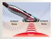
The same ambient noise that travels through the air also travels through the body. 3M's patented ANR technology cancels out both sources of ambient noise, leaving the critical body sounds that need to be heard.
